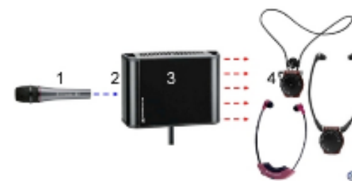
On picture: Infrared Systems
